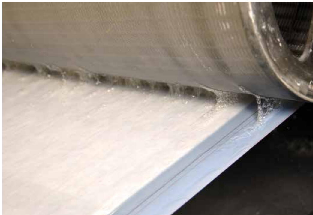
The dandy roll gives the paper a ribbed structure.
